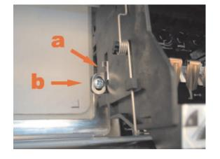
3. With a pair of long nosed pliers pull the cartridge release spring assembly (a) up and out of the carriage assembly. Not all Kiosk have a release spring assembly.
