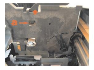
6. Slide the head plate (b) to the left until the right had side is free from the slot. Then lift the right side of the head plate up and towards the right to free it from the left had slot.
