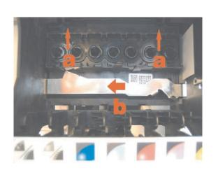
The head is angled up and away from the carriage, the cable can them be carefully unplugged. The metal cover indicated to by the arrow will be removed before replacing the print head.
