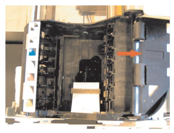
Once the guide has been removed the cable can be easily accessed to plug into the new head. The arrow is pointing to the porous pad that must be fitted when ever the head cable is replaced. This pad protects the head from being damaged by minor ink spills.
