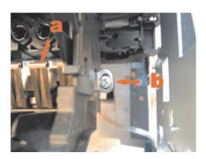
5. Gently depress the clip (a) so that the front portion of the head cable shield can be lifted free.
