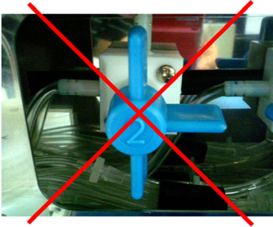
NG: Air gets into the tubes
