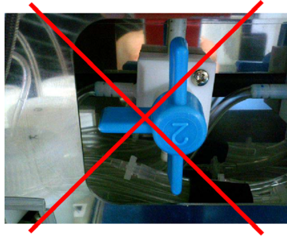
NG: Supplies both ink and cleaning liquid
